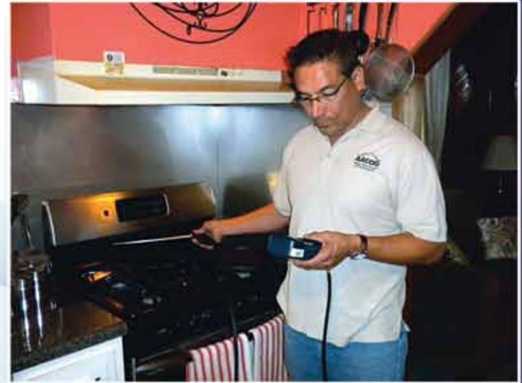
Weatherization Inspector Rick Morales testing the carbon monoxide levels on a client's stove using a Combustion Gas Analyzer.
