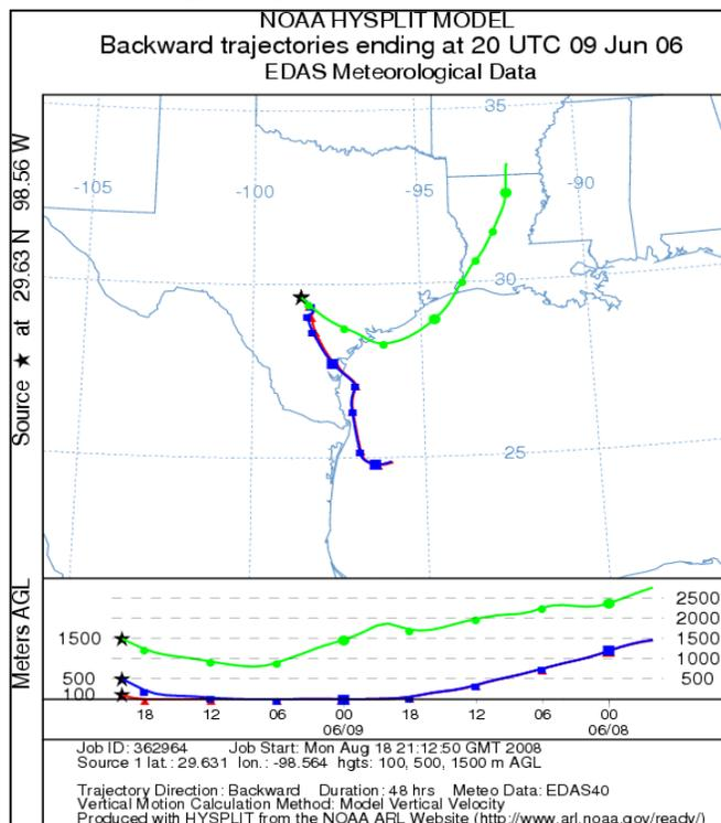
As displayed in the figures, back trajectories are split into 100 (red), 500 (blue), and 1,500-meter (green) elevations. The plots show that winds came from the southeast on these high ozone days at both the 100-meter and 500-meter elevations. By using the data represented in these figures, wind directions and emission source regions can be estimated.
