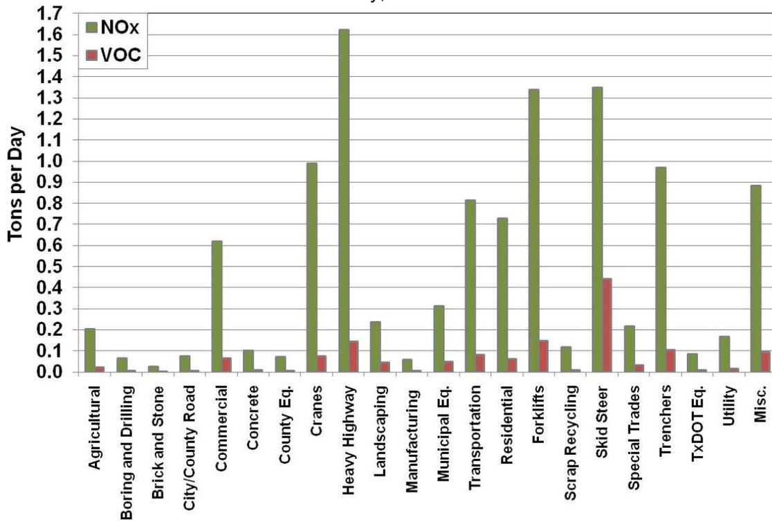
Figure 2-2: Construction Equipment Emissions by Equipment Type, Tons per Ozone Season Day, 2006
