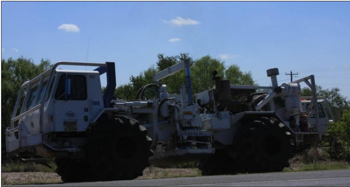
Figure 3-1: Seismic Survey Vibration Truck or Vibroseis Vehicle in the Eagle Ford shale play 81
