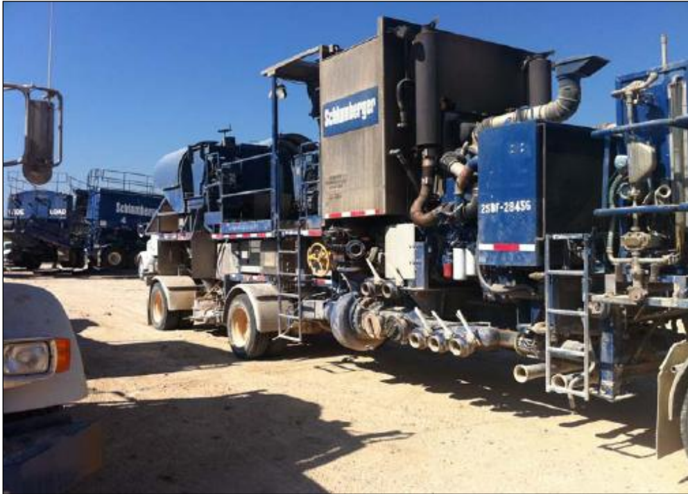
Figure 5-5: A Blender Truck used during Hydraulic Fracturing 263
