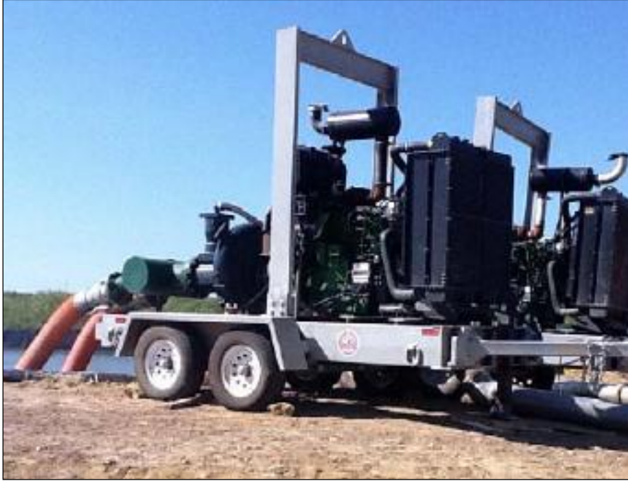
Figure 5-4: A Water Pump used during Hydraulic Fracturing 262
