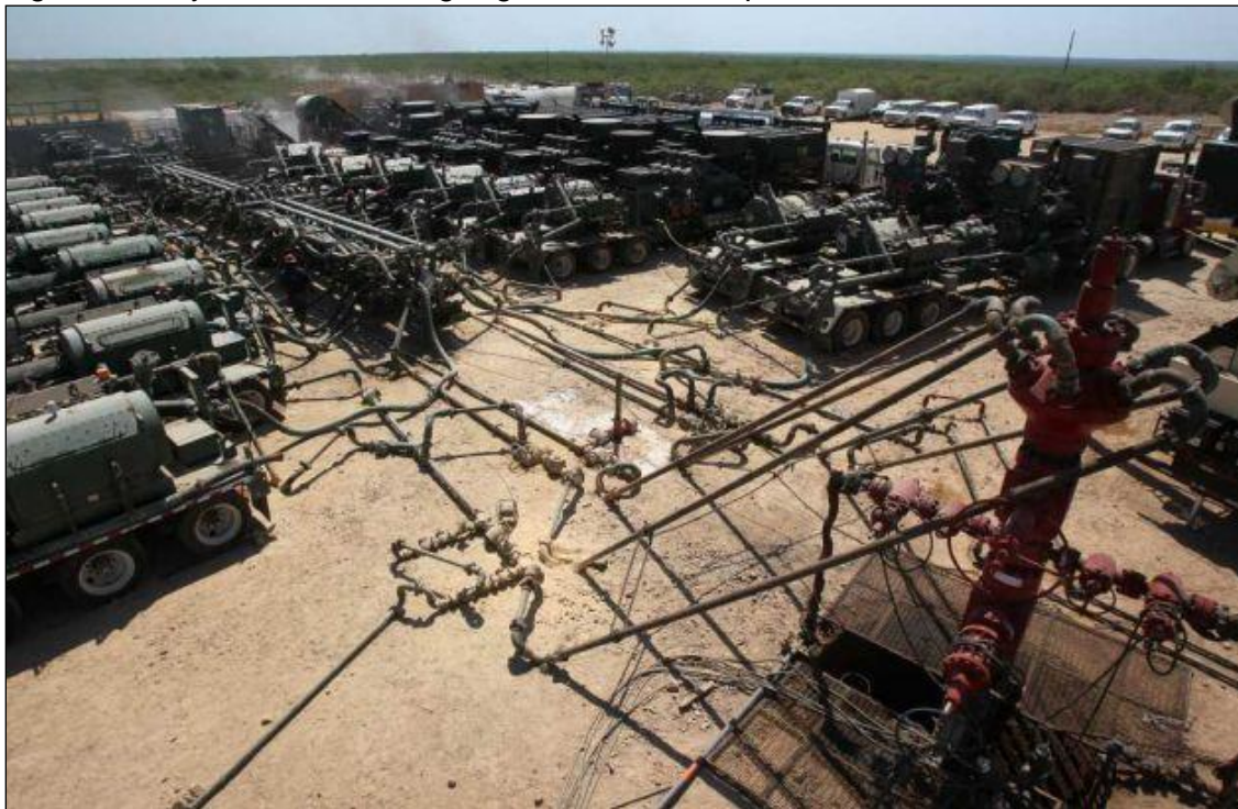
Figure 5-1: Hydraulic Fracturing High Pressure Pump Trucks 224
