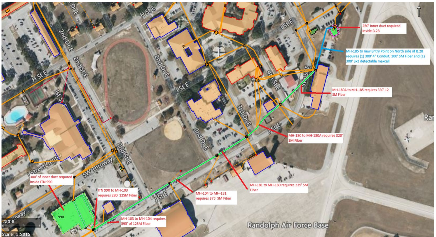
8.4 Figure 4: Fiber Optic Cable Route from Bldg. 990 to Bldg. 28
