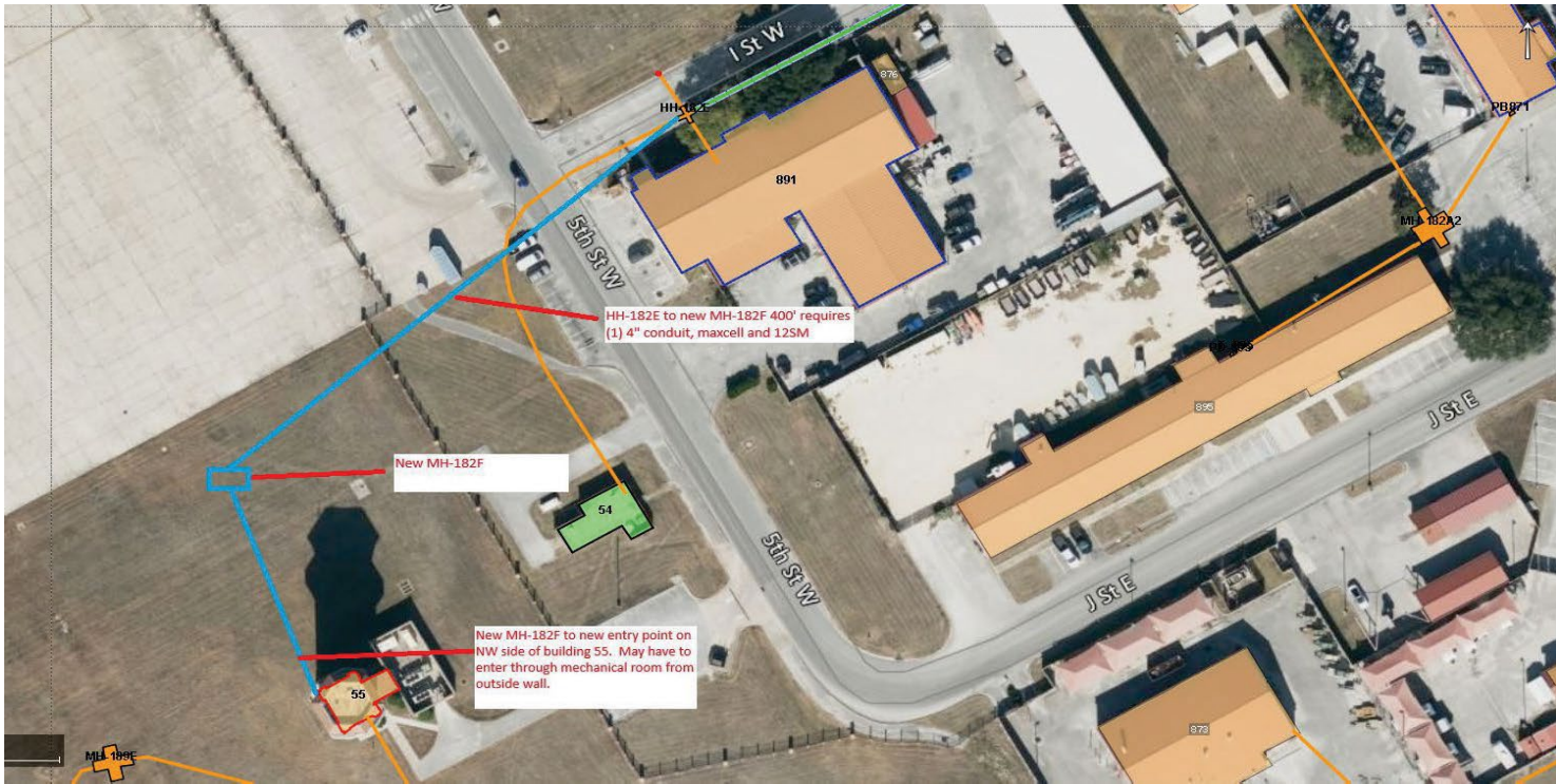
8.4 Figure 4: Fiber Optic Cable Route from Bldg. 990 to Bldg. 28
